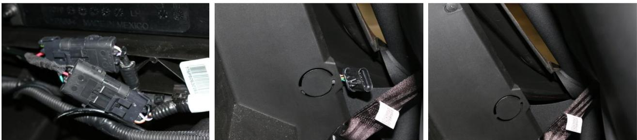
**Run the other end** - of the rear harness to the front kick panel. The plastic has a perforated circle behind the driver's seat or rear seat behind the driver on the MAX, at this location you can push the rear harness single connector through the plastic gap to the passenger compartment, follow the frame along the driver's side, the harness can be hidden in the side panels and goes up behind the removed kick panel over the frame rail.
