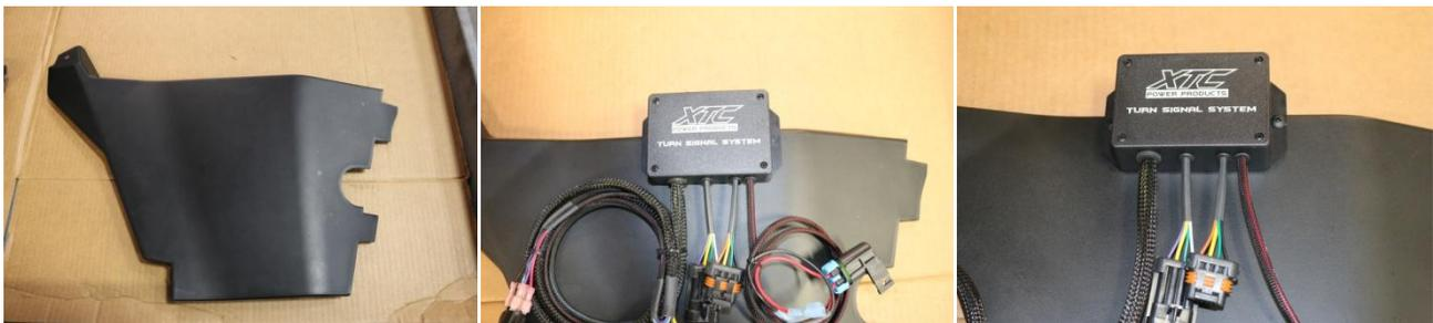
3. **Run the Rear Harness** - Starting at the rear drivers side light harness, these connections are on the plastic wall in the front engine area, take the end of the cable with two connectors on it and run it from the OEM Rear Light Harness on the Driver's side to the OEM Rear Light Harness on the Passenger side, follow the factory wiring, unplug both harness and install our harness into the factory harness. Secure using the supplied cable ties
