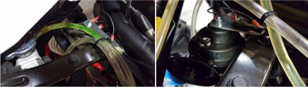
8. Run power wire to 12vdc accessory stud under the hood and ground the black wire.
