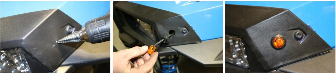
Run the short front harness through rubber grommet to the front right LED. Connect the green wire to the black and the white to white, continue harness to left LED, yellow wire attaches to black wire and the white wire goes to white. NOTE: Black wire is positive and will not work if reversed. White is ground. Secure the Harness using the provided cable ties.
