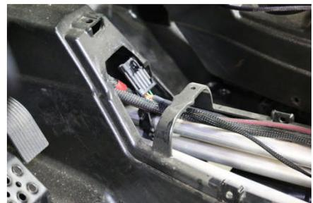
4. **Plug rear Harness into OEM Connector** - Unplug wire harness at rear left side and connect our harness, see photo below. (Note: There is a Red and Brown power wire provided for an optional license plate light). Run the rest of the harness to the rear lights, Green goes to right light and Yellow goes to Left. You may leave the factory rear harness in or remove it.
