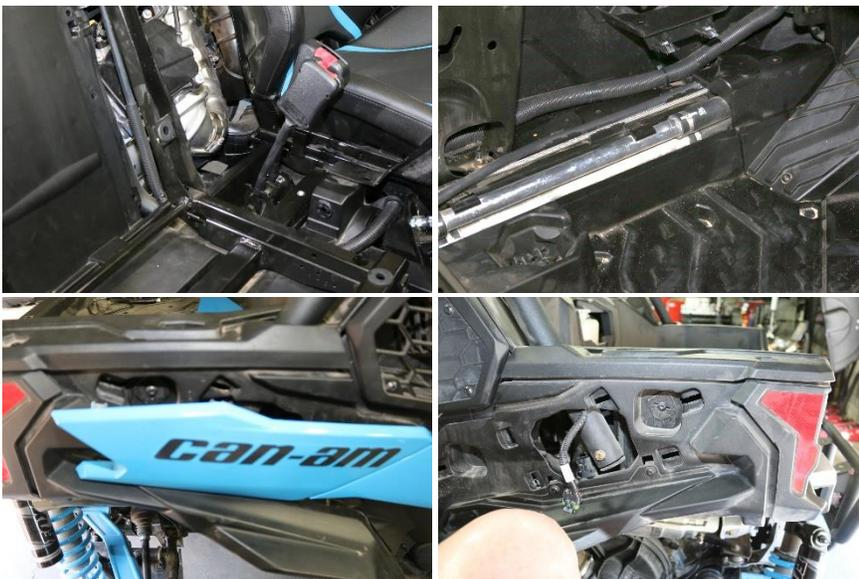
2. **Run the Rear Harness** – Un-roll the rear long harness, take the end with the one 4-way connector, starting in the center console at the seat belt mounts run it up to the front of the tunnel following the main OEM wire harness. Pull it through until the split for the right and left are at the rear of the center console.
