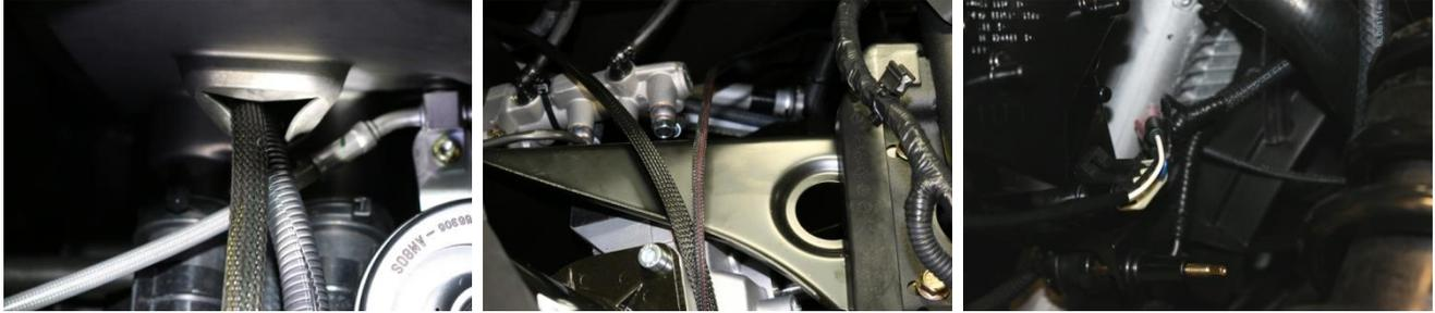
7. **Attach Front Harness to lights** - The Green and white wire go to the right/passenger side LED, attach the Green to the Black and the White to the White, the Yellow and white wire go to the Left/Driver side LED, attach the yellow to the Black and the white to the White (above right photo). NOTE: Black wire is positive and go to the Green and Yellow, they will not work if reversed. White is ground. Secure the Harness using the provided cable ties.
