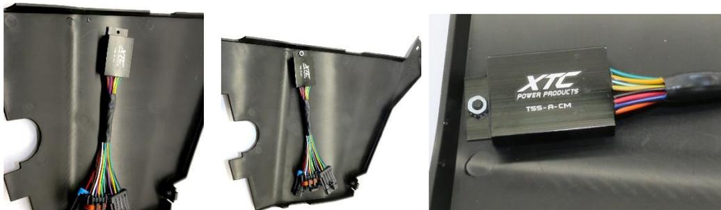
3. **Run the Rear Harness** - Starting at the rear driver's side light harness, these connections are on the plastic wall in the front engine area, take the end of the cable with two connectors on it and run it from the OEM Rear Light Harness on the Driver's side to the OEM Rear Light Harness on the Passenger side, follow the factory wiring, unplug both harness and install our harness into the factory harness. Secure using the supplied cable ties
