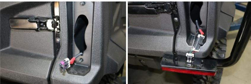
6. From the engine area run the long cable from the rear of the car to the front, keep it away from any **HOT or MOVING** parts. Take the 4-pin connector and run along the group of factory wires to the brake line. Follow the brake line to the center of the car under the seat, go across to the factory wiring and follow it to the fire wall and up to under the hood and plug into control module, secure the harness to the frame and brake line using the provided cable tie's.
