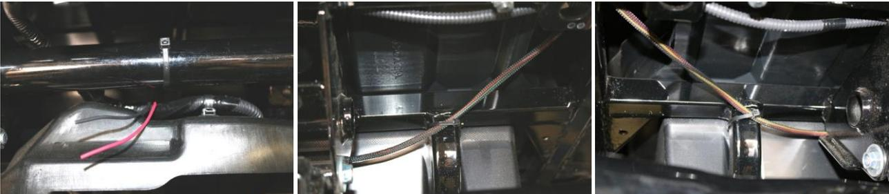
5. Plug the factory light connector into the new harness then plug into light and reinstall light, do the same for the other side.
