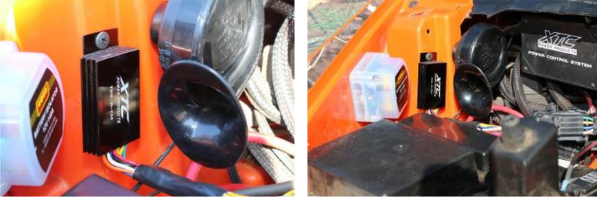
3. Drill a 3/8" hole in the side of the opening and mount the horn using the nut provided (shown above). Hook the violet wire and black ground wire to the horn terminals.
