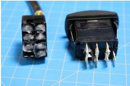
11. Install Horn/Hazard Switch - Using a new sharp razor, cut out a switch rectangle in the dash. Do not over cut, try inserting switch and trim as necessary. It helps to rock the razor to cut. Run connector through cutout and apply grease discussed above to the terminals on the Horn/Hazard switch and the connector and insert in panel.
