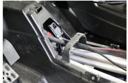
4. **Plug rear Harness into OEM Connector** - Unplug wire harness at rear left side and connect our harness, see photo below. (Note: There is a Red and Black power wire provided for an optional license plate light). Run the rest of the harness to the rear lights, Green goes to right light and Yellow goes to Left. You may leave the factory rear harness in or remove it.
