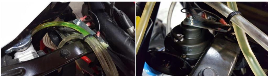
9. Run power wire to 12vdc accessory stud under the hood and ground the black wire.
