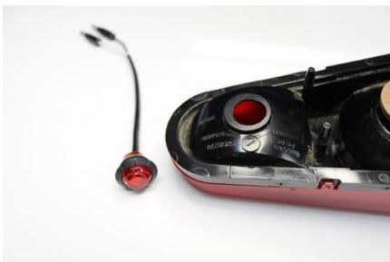
Sample: Rear LED Lights installed into an OEM rear Light Housing
