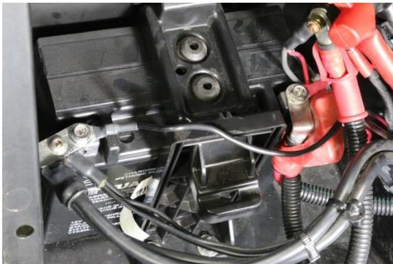
10. Run the Wire Harness with the two connectors through the center up to the radio and intercom mounting point.
