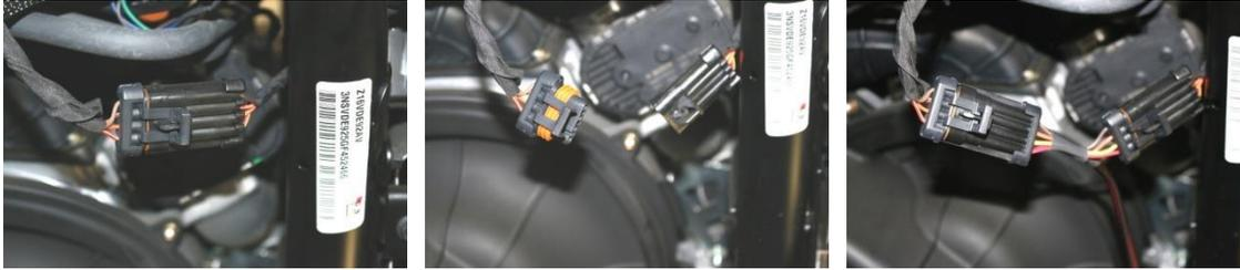
2. Plug the adapter into both OEM connectors as shown above.
