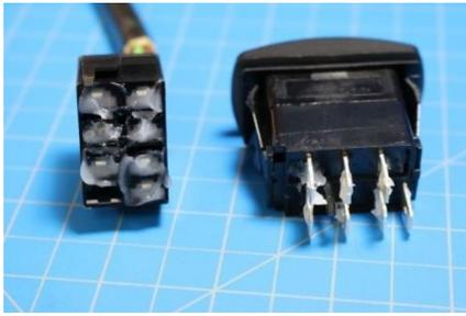
**Dielectric Grease** - LED flashers by design take very little current to activate. When water gets on the dash and lands on the top of the switch, it can trickle to the connector causing it to activate the flasher by using the switches LED indicator, the system will continue to operate and does not hurt the system, but will continue clicking until the switch terminals dry. Just like the OEM we recommend using Dielectric Grease on all switch
