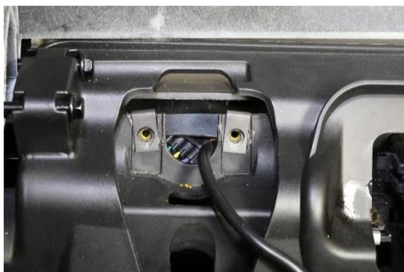
7. **Attach Front Harness to lights** - The Green and white wire go to the right/passenger side LED, attach the Green to the Black and the White to the White, the Yellow and white wire go to the Left/Driver side LED, attach the yellow to the Black and the white to the White. NOTE: Black wire is positive and go to the Green and Yellow wire, they will not work if reversed. White is ground. Pull any excess wire back under the dash and secure the Harness using the provided cable ties.
