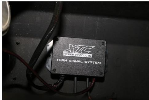
3. Unroll the long rear cable, unplug the rear light harness above the engine and plug our harness in-line, if TSS-POL-GBU it will be a 4-pin connector, TSS-POL-RCBU Ride Command system ordered then it will be an 8-pin Connector.
