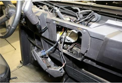
2. Mount the Control Unit as shown going through the switch plate opening using two self-tapping screws provided.
