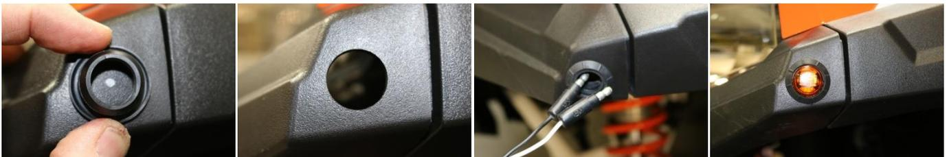
5. Plug the short Front Harness into the Control Box. Run the front right and left wire harness through the center grommet as shown, the green and white wire go to the right side of the car and the yellow and white go to the left side, connect the green wire to right black wire and yellow wire to left black wire and white to white on both.
