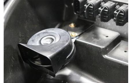
9. Install the Horn. Install the Horn mounting bracket to the horn. Pull out a Busbar Torx screw or using the included #10 x 1" screw, mount the horn in one of the plastic holes as shown above. Connect the violet wire to one of the horn terminals and the black wire to the other terminal.
