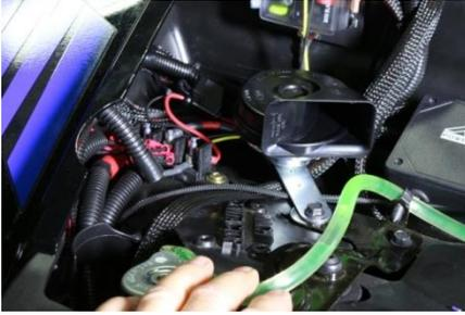
Connect the violet wire from the front harness to one of the horn terminals and the black wire provided to the other terminal.
