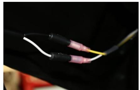
8. Lay the front small light harness out in the front under the hood, run the connector with the green wire to right side LED and run the connector with the yellow wire to the left side. Run the 4-pin connector through the hole in the fire wall to the control unit. Insert bullet connectors into LED connectors as shown above. **NOTE: The Black LED wire is positive and**
