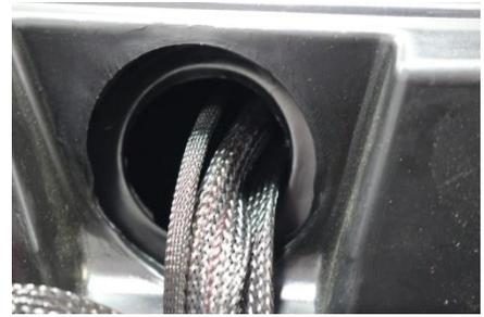
5. Plug the new Harness into the rear OEM light connector and run the Green wire with plug to the right side rear tail light and the Yellow wire with plug to the left tail light, use the existing cable holds to attach replacement harness. Reinstall tail lights.
