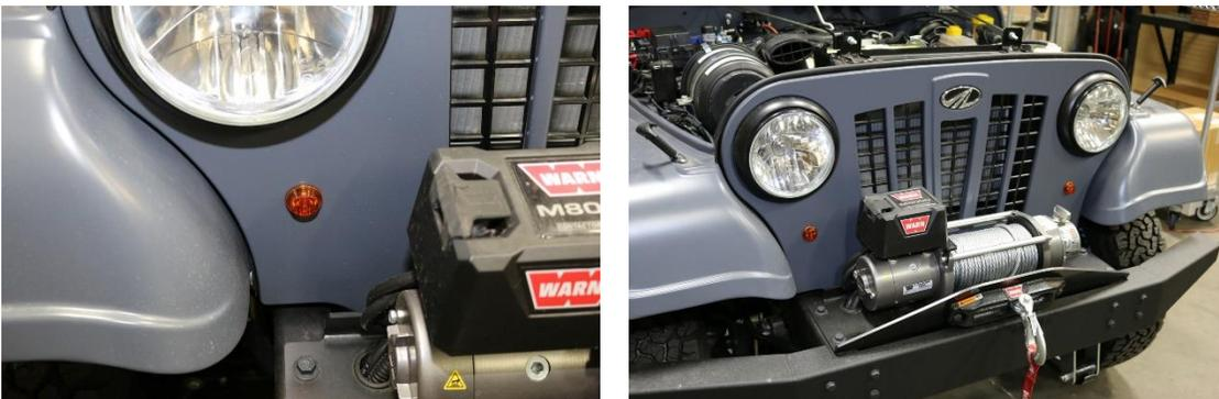
7. Lay the front small light harness out in the front under the hood, run the connector with the green wire to right side LED and run the connector with the yellow wire to the left side. Run the 4-pin connector through one of the rubber grommets in the fire wall to the control unit. Insert bullet connectors into LED connectors as shown. **NOTE: The Black**
