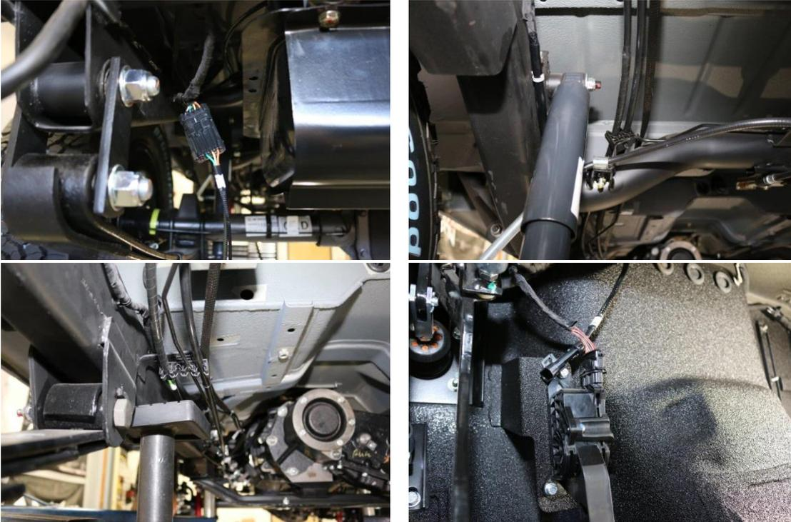
5. Mount the Control Unit under the grommets using two self-tapping screws provided and Plug the Rear Harness in.
