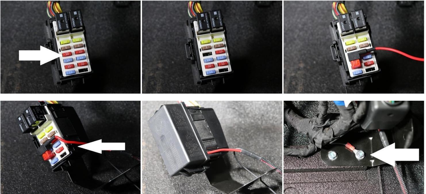
Run the power wire down the slot on the right side and reinstall the fuse cover. Remount the fuse box and using the mounting screw attach the black ground wire as shown.
