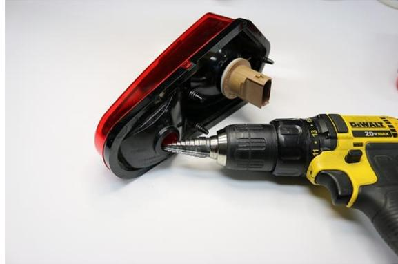
Slide rubber grommet off the LED, insert LED through the hole with wires coming out, then install rubber grommet into hole making sure wire comes through the grommet, using soapy water in the grommet, pull the LED light back through the grommet. If it seems to tight drill out holes out to 13/16".
