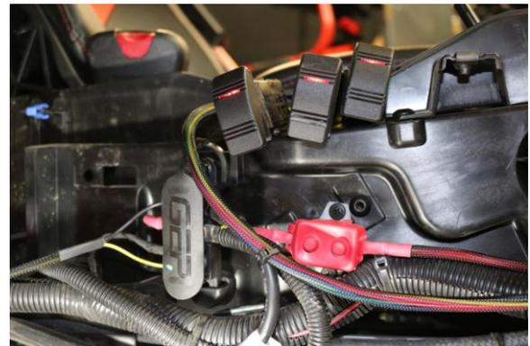
9. Run the power wire from the fuse block to the factory busbar fulltime power( Center Stud), secure the 50 amp Circuit Breaker with the supplied screws.
