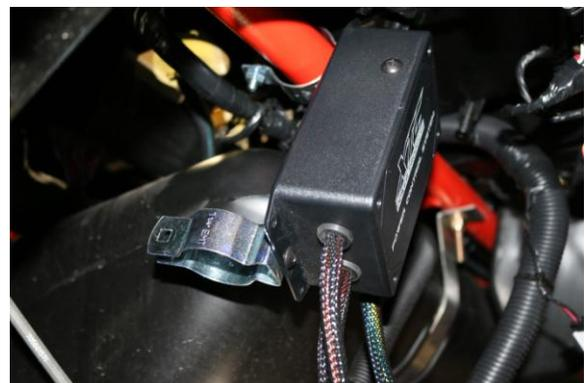
Tighten the first clamp up as much as possible before sliding the unit further over and setting the second clamp to make it easier to do the final tightening.
