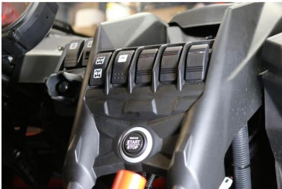
8. Run the other switches down to the left drivers side or center console below where the cup holder are. Attach the yellow wire to the switched bottom stud and the black wire to the top ground stud on the factory busbar
