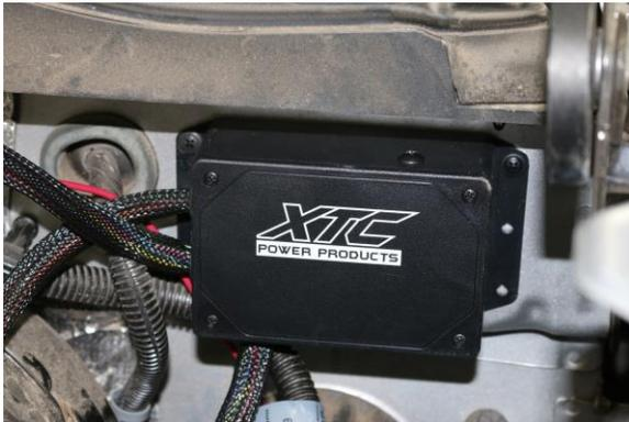
**STEP 2** Mount Fuse box on fire wall, make sure it is mounted where it can be accessed to replace fuses.
