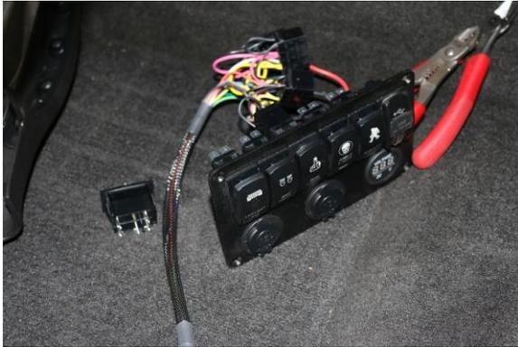
**Step 5** Run the long wire harness with the **terminals that were compressed with Heat Shrink** through the fire wall to the switches.
