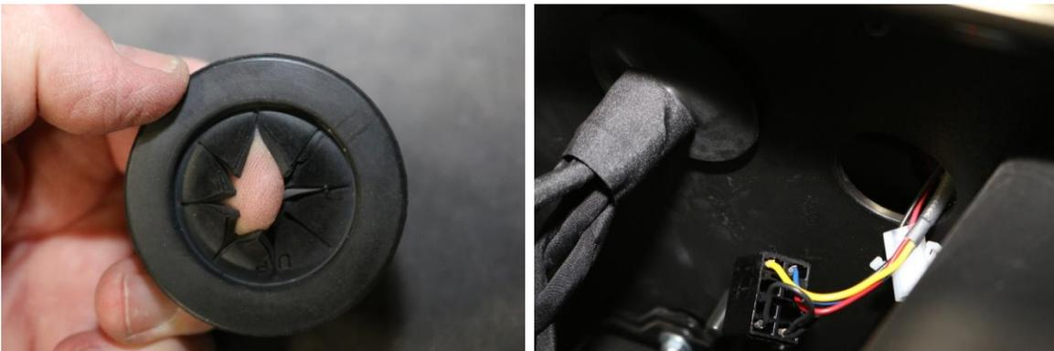
4. Using the switch mount as a template cut the dash for the switch. Make sure there is room behind the dash for the Switch and Harness
