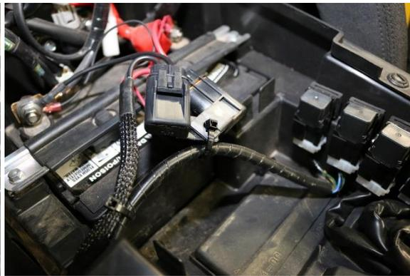
7. If not done in step 2, remove the screw from the Negative Black Terminal of the battery and make sure to push it to the side.
