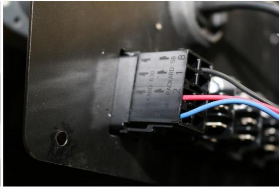
5. Run the Switch connector to the switch and plug in.
