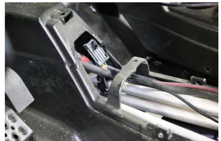
4. **Plug Rear Harness into OEM Ride Command 8 pin Connector** - Unplug wire harness at rear left side and connect our harness, see photo below. (Note: There is a Red and Brown power wire provided for an optional license plate light).
