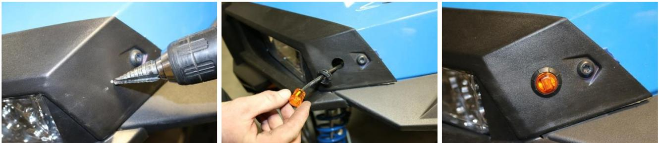
Run the short front harness through rubber grommet to the front right LED. Connect the green wire to the black and the white to white, continue harness to left LED, yellow wire attaches to black wire and the white wire goes to white. NOTE: Black wire is positive and will not work if reversed. White is ground. Secure the Harness using the provided cable ties.
