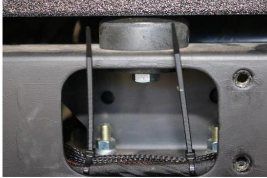
4. Unroll the long rear cable, plug it into the rear harness just installed. Run the cable under the chassis up through one of the rubber grommets that was cut. Secure the harness using the supplied Cable Ties.
