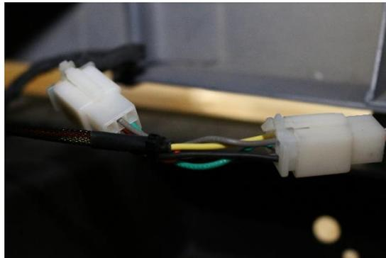
3. Run the other side of the Harness through the bumper over to the passenger side and plug in-line. Secure with cable ties.
