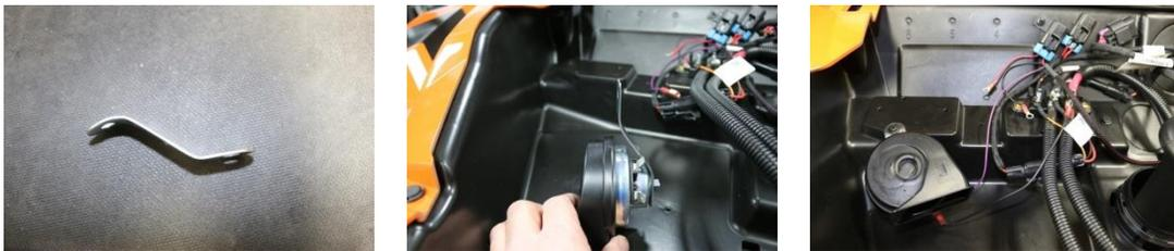
Connect the violet wire to one of the horn terminals and the black wire provided to the other terminal, run the black wire over to Buss Bar and attach to ground. If the car has not been upgraded with the Buss Bar Power Up Kit or Winch Kit, then the black wire will need to be grounded to the buss bar mounting screws
