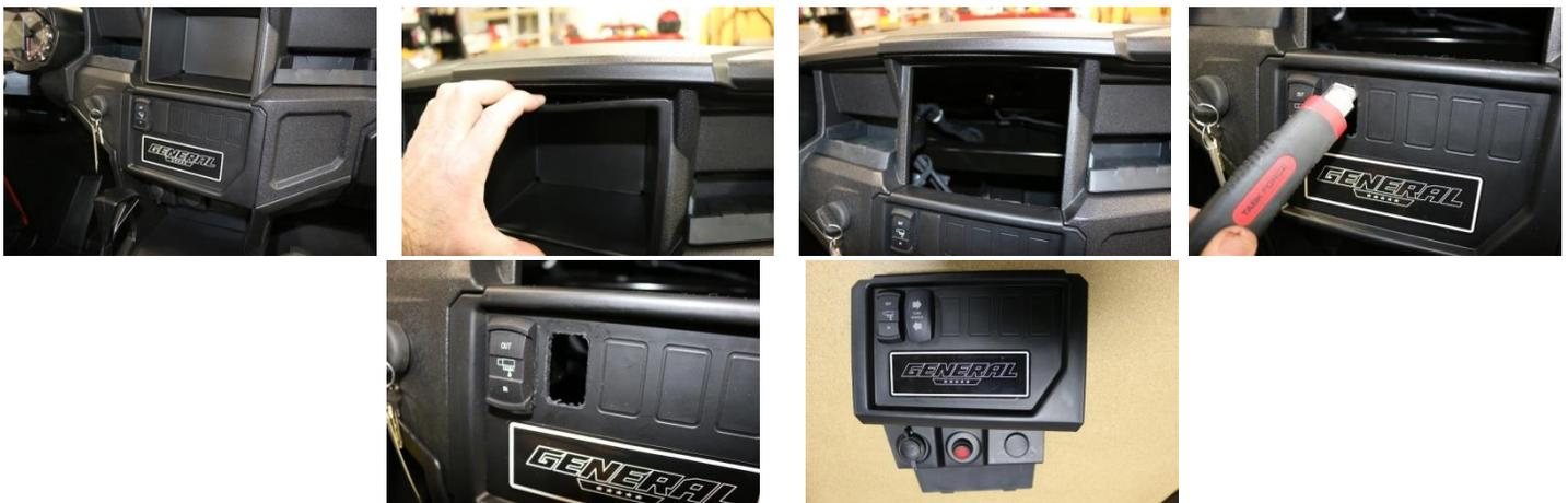
8. Run Switch Harness - Push the 10 pin Horn connector through the grommet in center, then push the 8-pin Turn switch connector through. Note: The grommet can be removed and stretched over the switch connector and reinstalled. Run the connectors through the rectangle switch cutouts and use included grease (see step 9) then connect to turn switch and slide switch into dash as shown.
