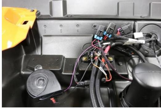
**(Note: The car does not have ground hooked on any of the studs under the hood unless the Bus Bar Power Up kit or Winch kit are installed, the first stud is keyed 12vdc, second stud is ground if wired and the third stud in battery direct if installed, **but no fuse or circuit breaker**. You must run a ground wire from the chassis to the ground stud or run our black ground wire directly to the chassis for a ground if upgrade is not installed)**
