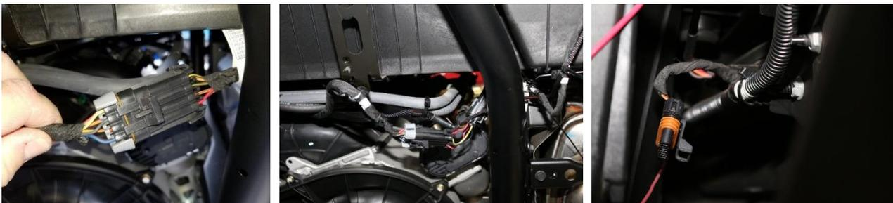
4. **Run Rear Harness** – Remove the seats and center plastic console. Starting at the rear run the long harness with the single 4 Pin Connector through the center of the car up the outside of the firewall through the rubber grommet to the control box and plug in. **Secure cable using the supplied cable tie's making sure to keep the harness away from any Hot or Moving parts.**
