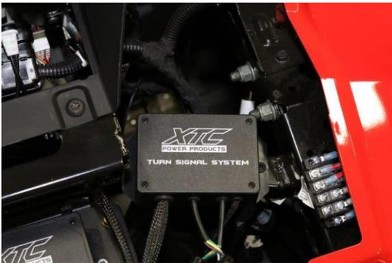
3. **Plug Rear Harness into OEM Ride Command 8 pin Connector** - Unplug wire harness at rear left side and connect our harness inline. (Note: There is a Red and Brown power wire provided for an optional license plate light). Reach into the rear and unplug the center brake light, run the 4-pin connector to the third brake light and plug in.
