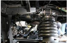
Using the provided cable ties secure the harness to the frame.
