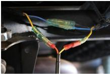
Run the Green wire to the right-side tail light, go over the heat shield and unplug the yellow wire from the right tail light harness and plug it in. **NOTE: Drill two holes in the plastic on both sides above the heat shield and use a cable tie to hold the wire harness up from the sharp edge of the heat shield.**
