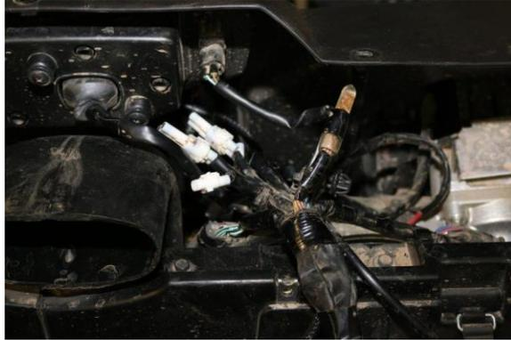
10. **Run Power Wire** – Run the power wire with the fuse over to main wire harness, under the dash there is accessory connectors for optional products, remove one of the white caps that does not have any wires coming out and plug the connector in to the factory wire harness. Reinstall Firewall. Leave the fuse on outside of the firewall when reinstalled.
