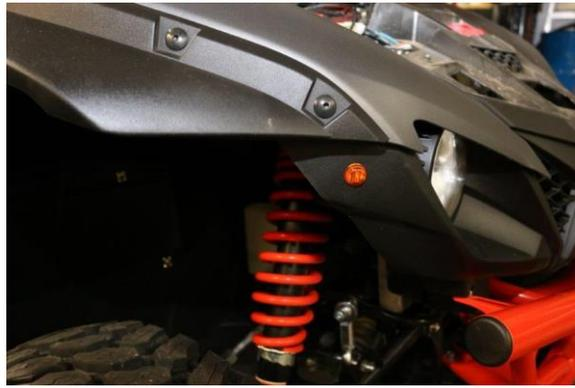
7. **Plug front Harness into control box.** Run the Green wire harness to the right/passenger side and the yellow wire harness goes to the left/driver's side. Both green and yellow wires are positive and go to the black wire on the LED Light, the white wire goes to white. Secure the harness with the provided cable ties. **NOTE: Black wire is positive, and the White is ground, they will not work if reversed.**
