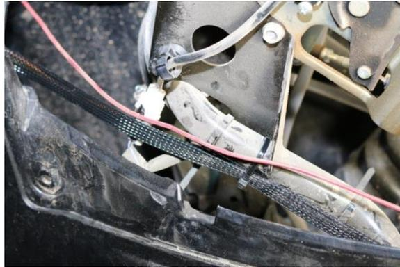
**WARNING! Verify that there is clearance before drilling the holes for the LED's and keep the harness away from any hot or moving parts.**
