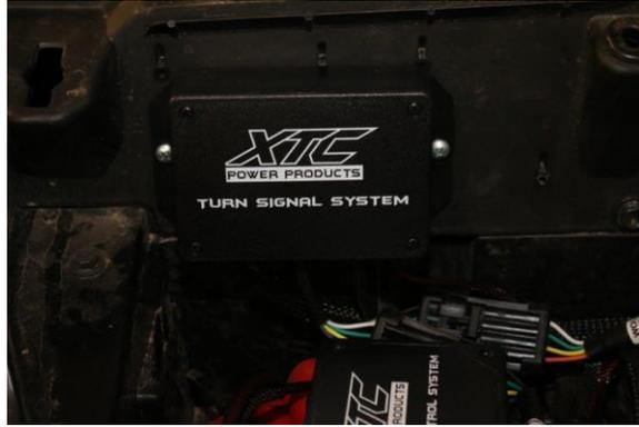
5. **Run the Rear Harness** - Attach the long extension harness to the previously installed rear light harness. Run the rest of the harness with the male four pin connector through the center of the car, through the fire wall at the main wire harness up to the control box and plug into the mating connector, **make sure to keep the harness away from any hot or moving parts, secure with provided cable ties.**
