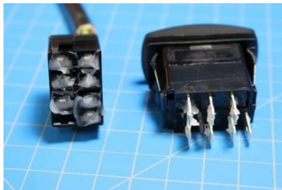
**Dielectric Grease** - LED flashers by design take very little current to activate. When water gets on the dash and lands on the top of the switch, it can trickle to the connector causing it to activate the flasher by using the switches LED indicator, the system will continue to operate and does not hurt the system but will continue
